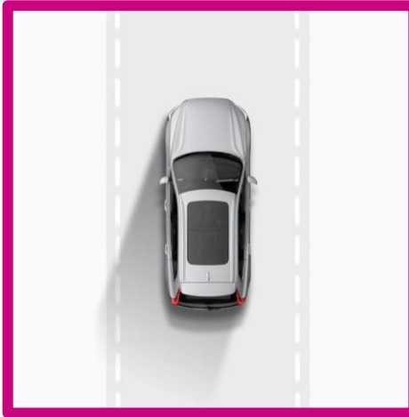
Run-off road mitigation 65-140 kph
