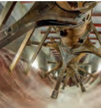
Paddle mixer unit in Dry Fermentation System
